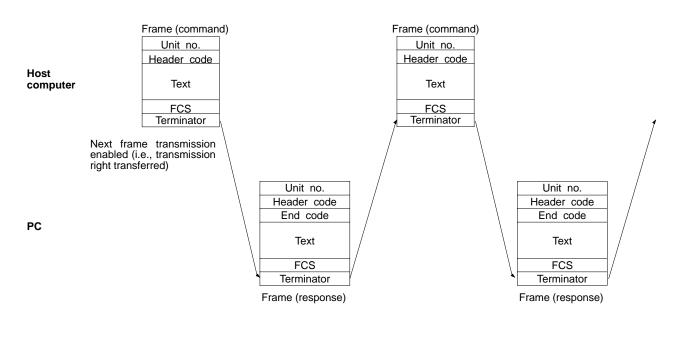
**Commands from PC** It is also possible in host link communications for the PC to send commands to the host computer. In this case it is the PC that has the transmission right and initiates the communications.
